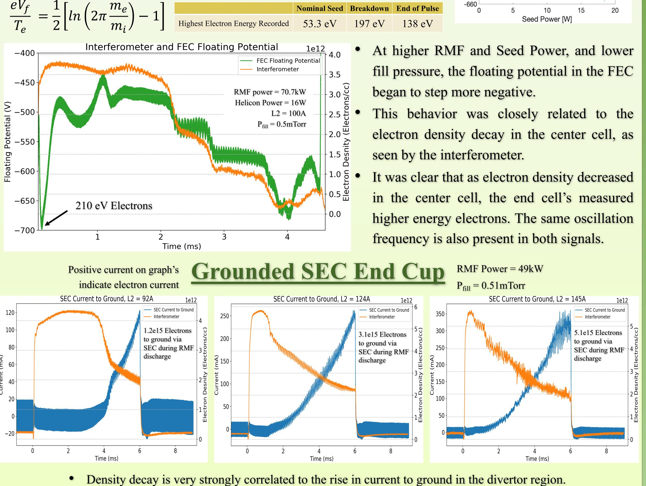
• The same oscillation frequency ( $\approx 13$  kHz) present in the density decay is seen on the current.
